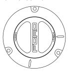
sure that each hub is fully engaged and that both hub locks are set to the same position (both set to LOCK or both set to FREE). To engage LOCK, turn the hub locks completely clockwise; to disengage the hubs (FREE), turn the hub locks completely counterclockwise.
